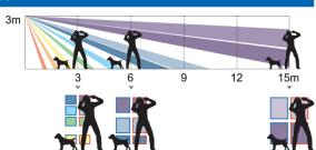
FMX has 78 dense zones to cover the whole detection area. At any spot within the detection area more than 4 (quad) zones are utilized to verify if it should generate alarm or not. Also The CORE platform enables the QUAD ZONE LOGIC to evolve to the next step. providing digital quantification of infrared energy, FMX enhances accuracy in both human detectability and pet immunity.
