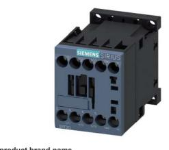
Power contactor, AC-3 12 A, 5.5 kW / 400 V 1 NO, 24 V AC, 50 / 60 Hz 3-pole, Size S00 screw terminal
