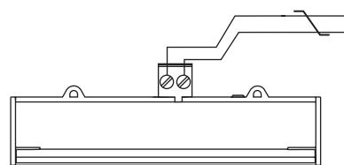
**en** The Lon and M-Bus ports are polarity-independent.
