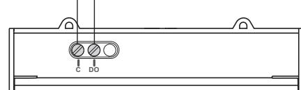
**en** The digital output is polarity-independent.
