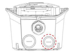
2. Remove the water proof cap and pass through the signal cable with appropriate conduit or cable gland.
