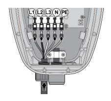
Install the copper wire as described. The section of copper wire connected to terminal shall be reserved enough tolerance to prevent any tension or stress from the external force.
