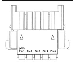
3. Connect the signal cable according to pin definition (2.2.7.1) and must connect to the Pin 1 (+5V).
